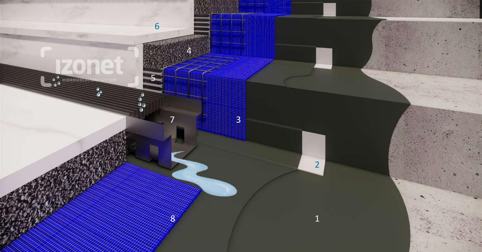
1. ARDEX 8+9 waterproof layer 2. ARDEX SK 12 tape 3. AQUADRAIN® SD drainage layer 4. ARDEX A10 + ARDEX QUARZKIES ME granulation 3.0 - 5.6 mm
