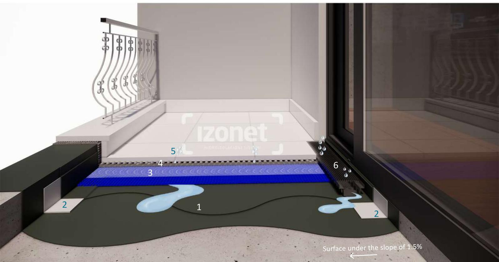
1. ARDEX 8+9 waterproof layer 2. ARDEX SK 12 tape 3. WATEC DRAIN KP+ drainage layer 4. ARDEX FB 9 L adhesive for stone/ceramic
