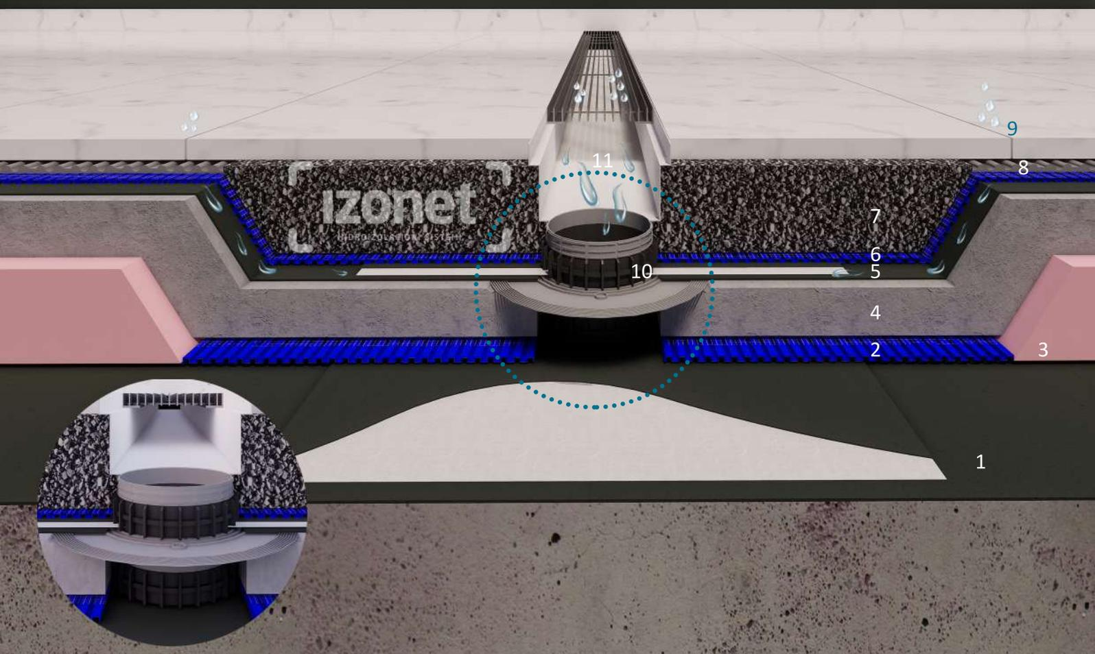
1. ARDEX 8+9 waterproof layer 2. WATEC® DRAIN KP+ drainage layer 3. XPS thermal isolation 4. cement screed 5. ARDEX 8+9 waterproof layer
