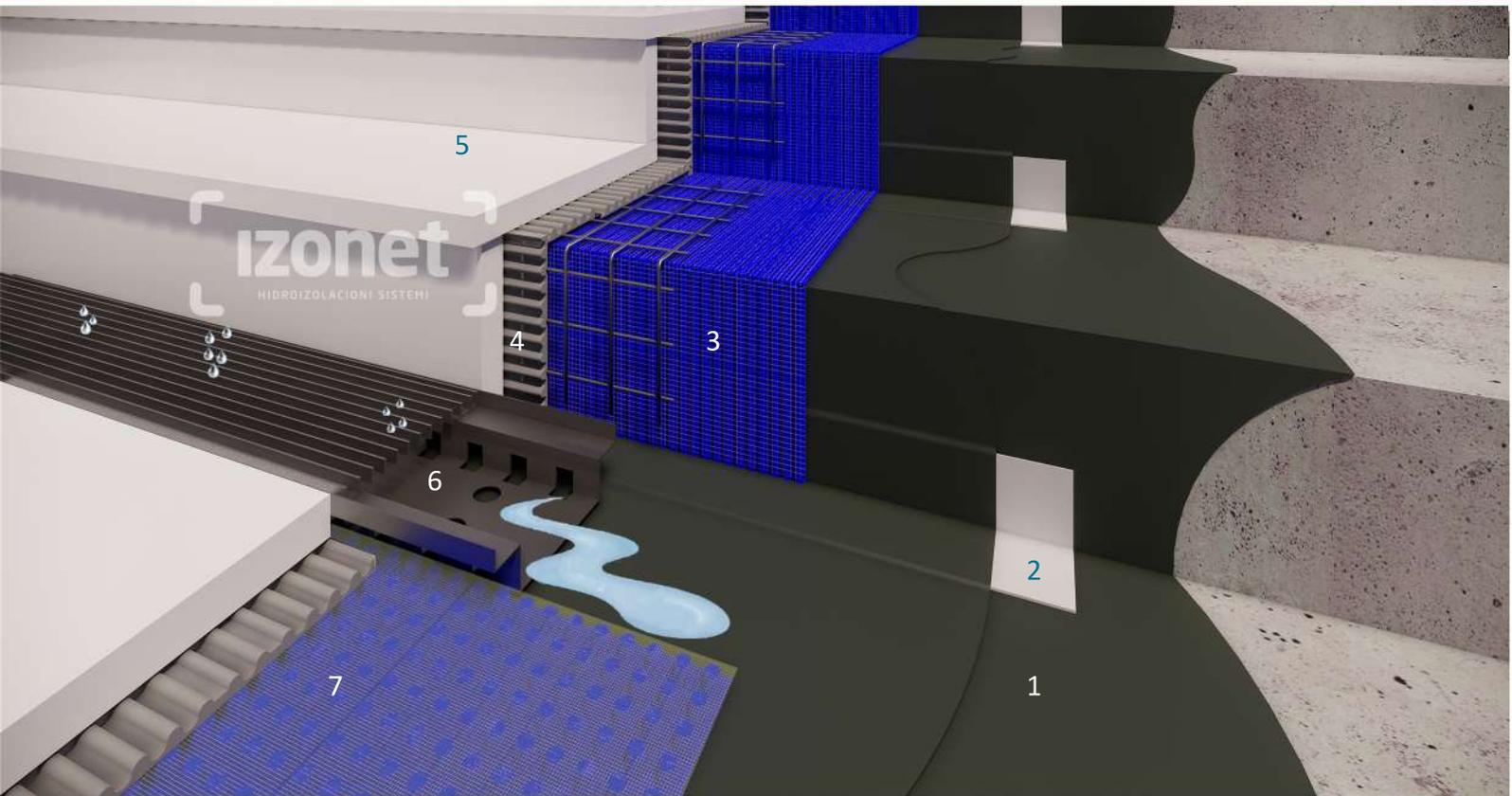
1. ARDEX 8+9 waterproof layer 2. ARDEX SK 12 tape 3. AQUADRAIN® SD drainage layer 4. ARDEX FB 9 L adhesive for stone/ceramic
