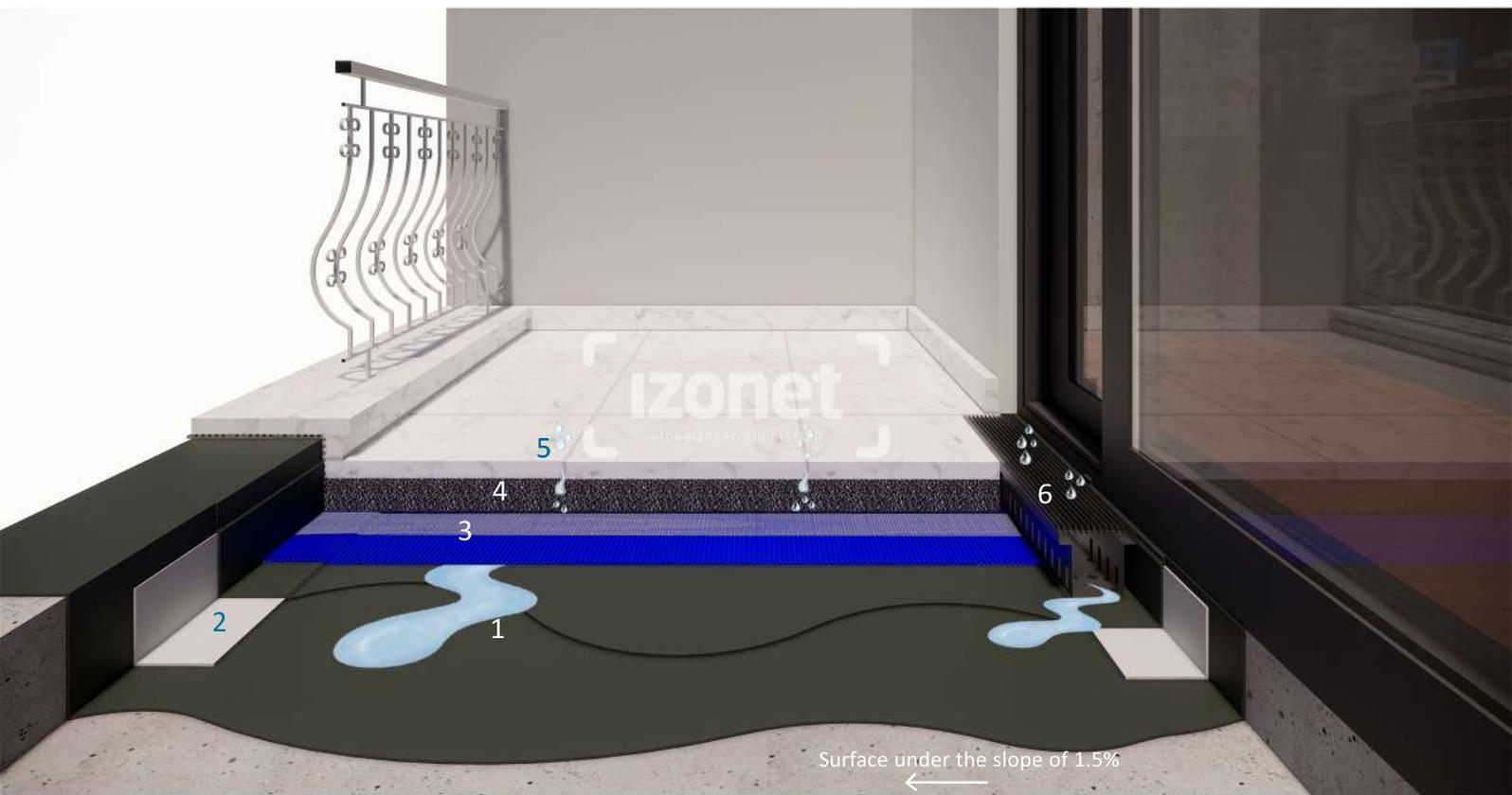
1. ARDEX 8+9 waterproof layer 2. ARDEX SK 12 tape 3. AQUADRAIN® EK drainage layer 4. ARDEX A10 + ARDEX QUARKIES ME granulation 3.0 - 5.6 mm
